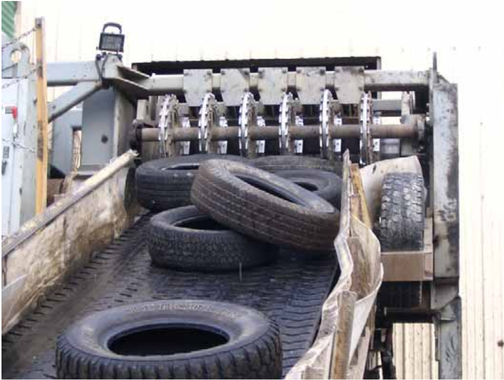
Figure 8.14 - Rimless casings in the process of shredding
