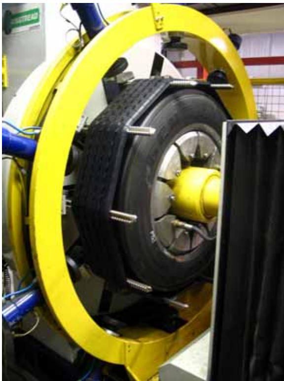
Figure 2.23 – Precured Tread (Unbroken) Brought Into Place around Casing (Ring-Tread Process)
