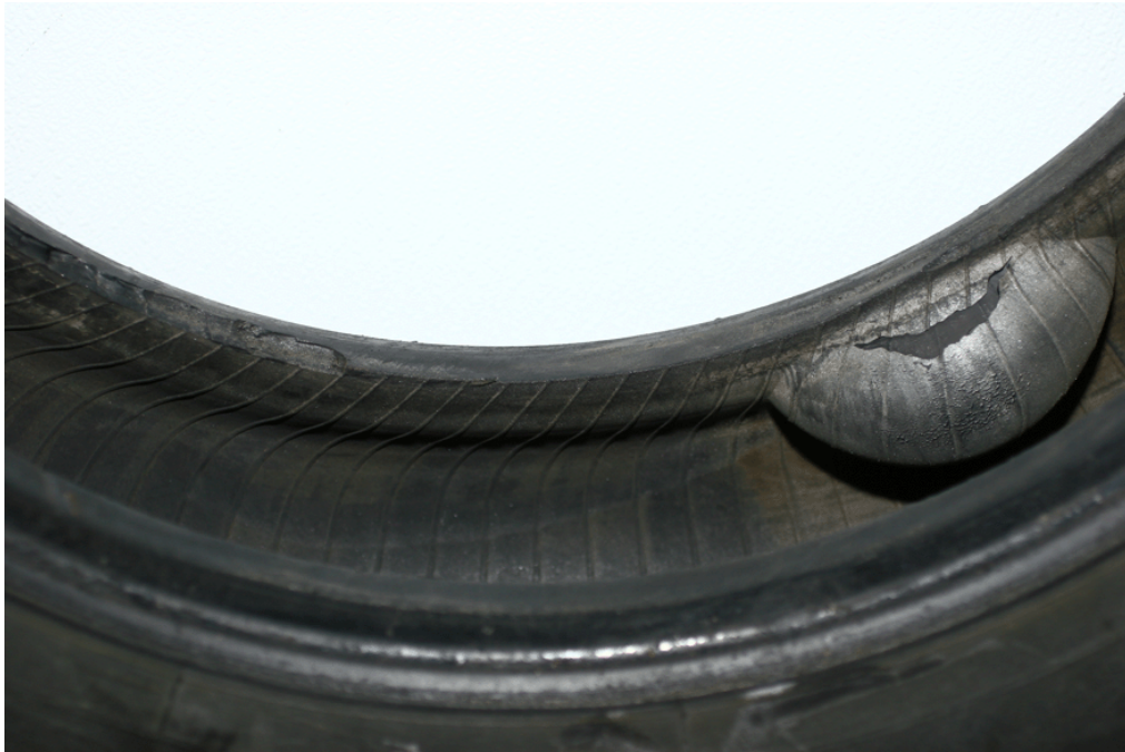
Figure 9.20- Excessive Intra-carcass Pressurization #1 - Separation as a result of excessive intracarcass pressurization
