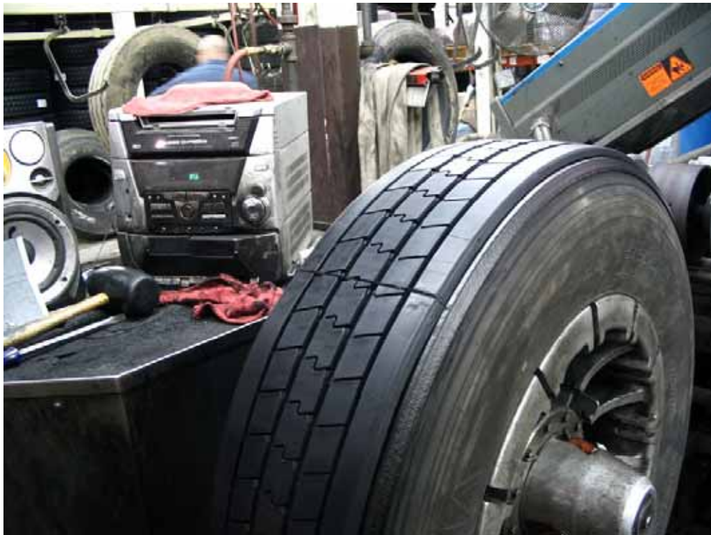
Figure 2.21 – Precured Rubber Tread Wrapped Around Casing (Precure Process) (Note: Tread splice is clearly seen)
