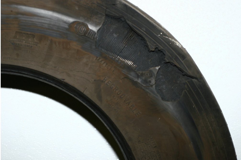
Figure 9.9 - Road Hazard #2 - Pinch shock damage. Sidewall separation resulting from excessive intracarcass pressurization, allowed by the pinch shock injury
