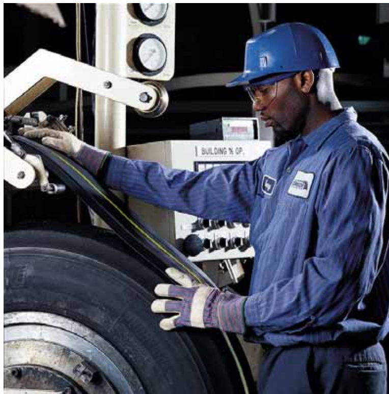
Figure 2.18 – Uncured Rubber Wrapped Around Casing (Mold-Cure Process) Courtesy of Bridgestone Firestone
