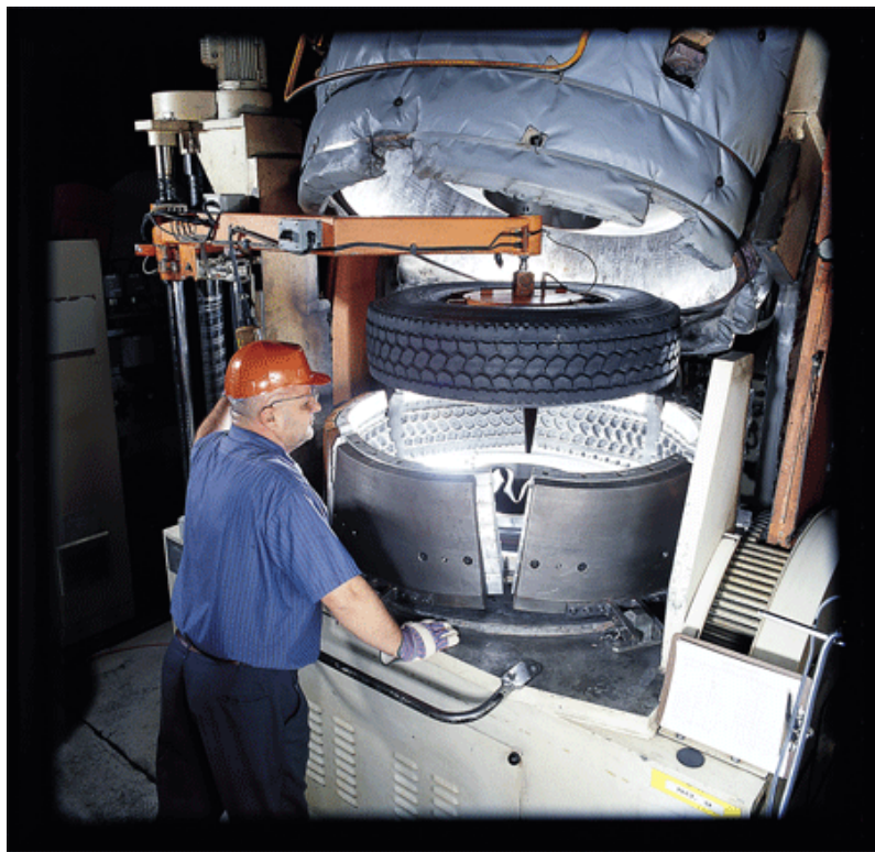
Figure 2.19 – Removing Casing from Retread Mold (Mold Cure Process)
