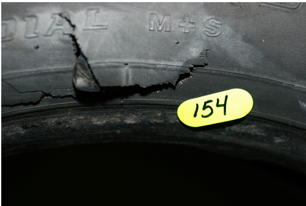
Figure 9.21 - Excessive Intra-carcass Pressurization #2 - Separation as a result of excessive intra carcass pressurization
