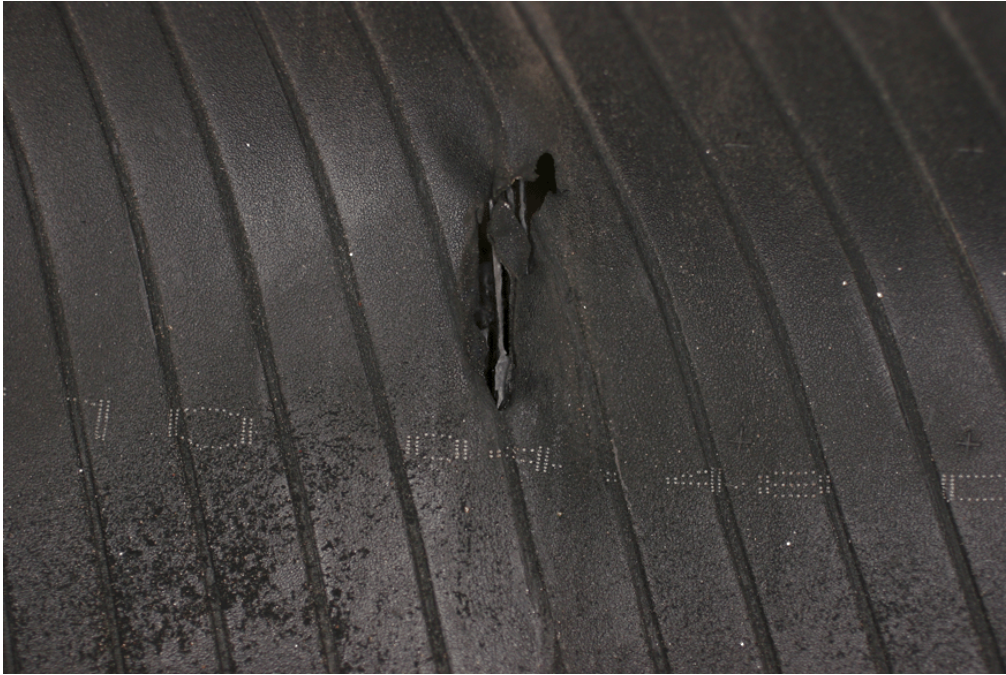
Figure 9.8 - Road Hazard #1 - Pinch shock damage. Sidewall separation resulting from excessive intracarcass pressurization, allowed by the pinch shock injury
