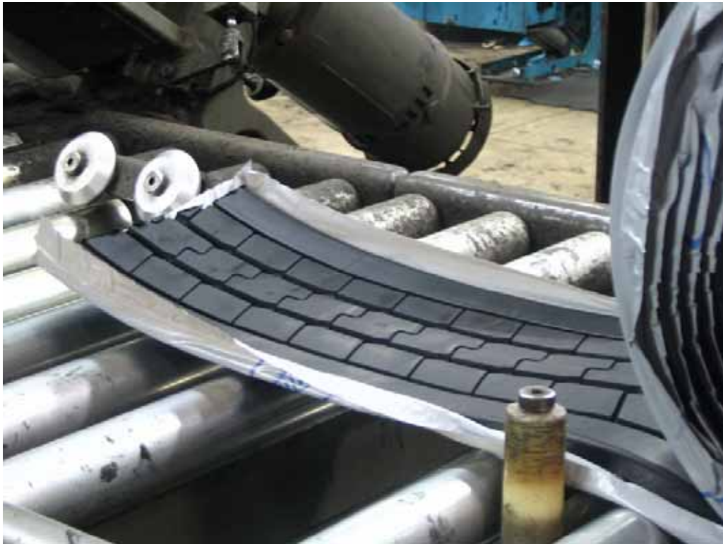
Figure 2.20 – Precured Rubber Tread (Precure Process)
