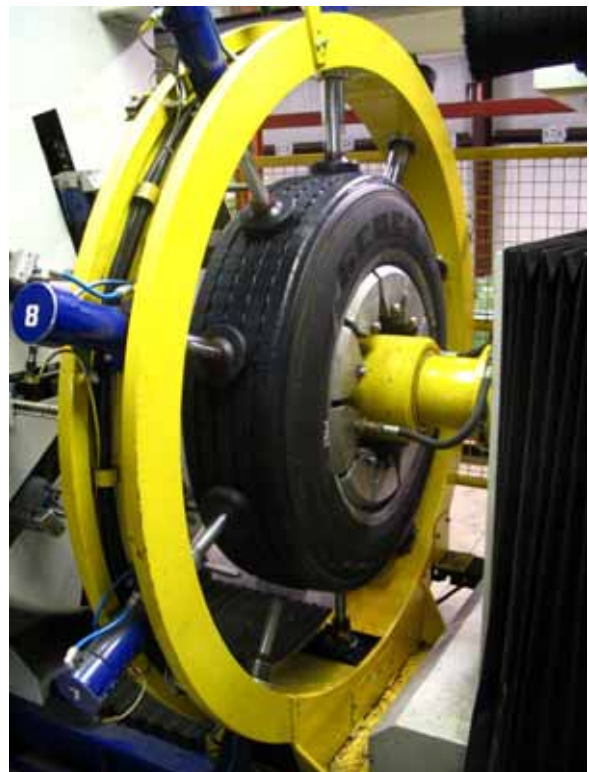
Figure 2.24 – Precured Tread (Unbroken) Positioned Into Place Around Casing (Ring-Tread Process)
