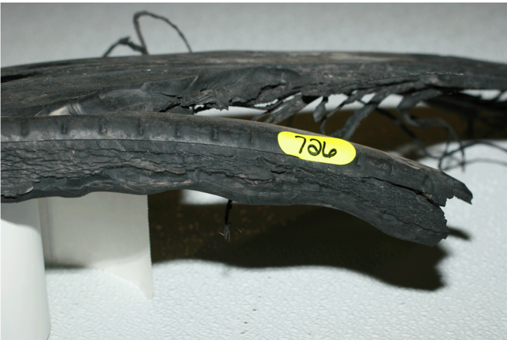
Figure 9.19 - Manufacturing/Process Issues #5 - Tire may have been unsuitable for retreading (severe weather cracking)
