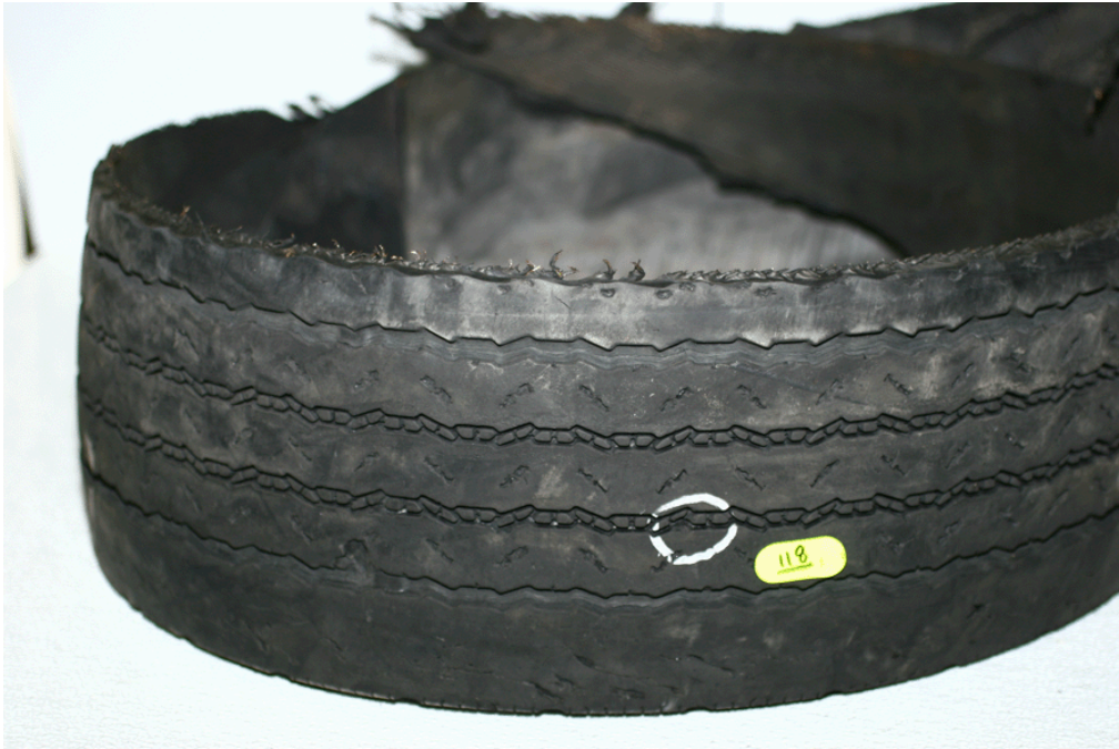
Figure 9.10 - Road Hazard #3 - Unrepaired crown puncture in original tread
