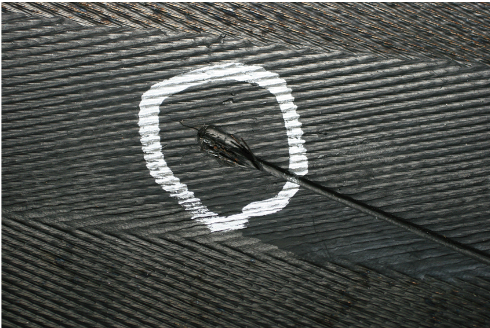
Figure 9.11 - Road Hazard #4 - Unrepaired crown puncture in original tread
