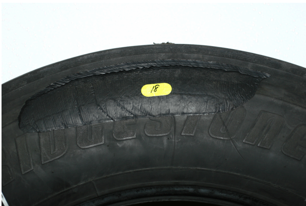
Figure 9.13 – Maintenance/Operational #2 - Use of improper (outside-in string plug) repair. Resulted in excessive intracarcass pressurization, sidewall separation, and tire failure
