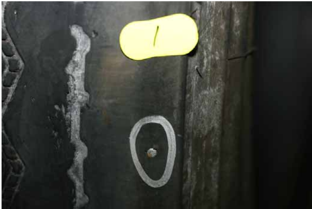
Figure 9.2 - Overdeflected Operation #1 - Apparent nail in outer rib, resulting in slow air loss and flex fatigue damage
