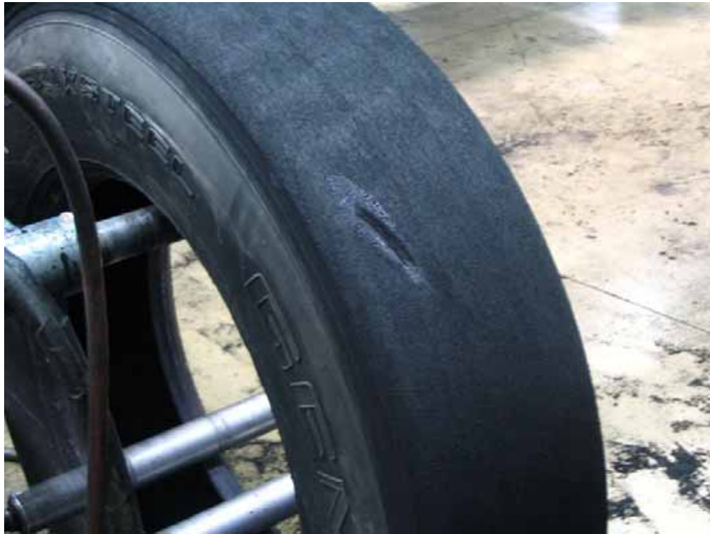
Figure 2.9 – A Buffed Casing Showing Area in Need of Repair
