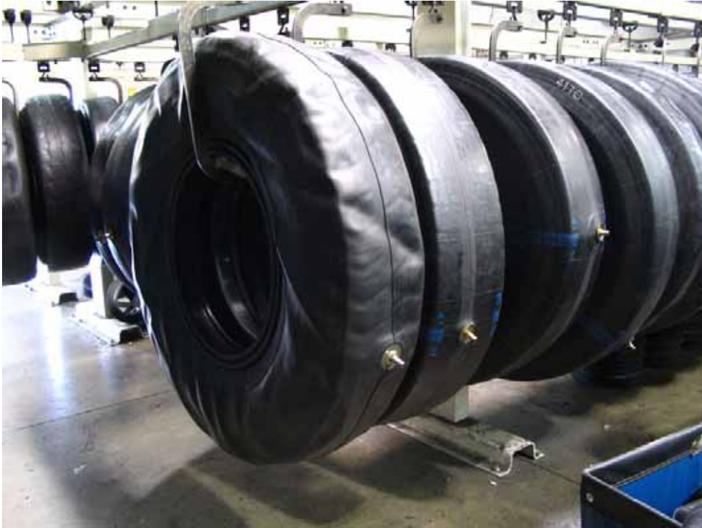
Figure 2.13 – Pre-Cured Retread Casings Enveloped
