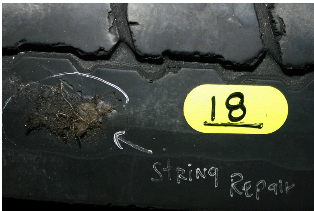
Figure 9.12 – Maintenance/Operational #1 - Use of improper (outside-in string plug) repair. Resulted in excessive intracarcass pressurization, sidewall separation, and tire failure
