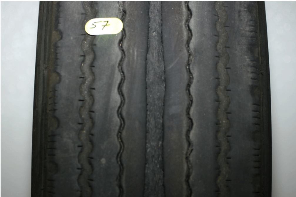
Figure 9.15 - Manufacturing/Process Issues #1 - Retread rubber separated at buff line. This resulted in a "raised" section of the tire's circumference. Localized, accelerated wear (9" in the center of the tread) resulted, extending to the buff line.
