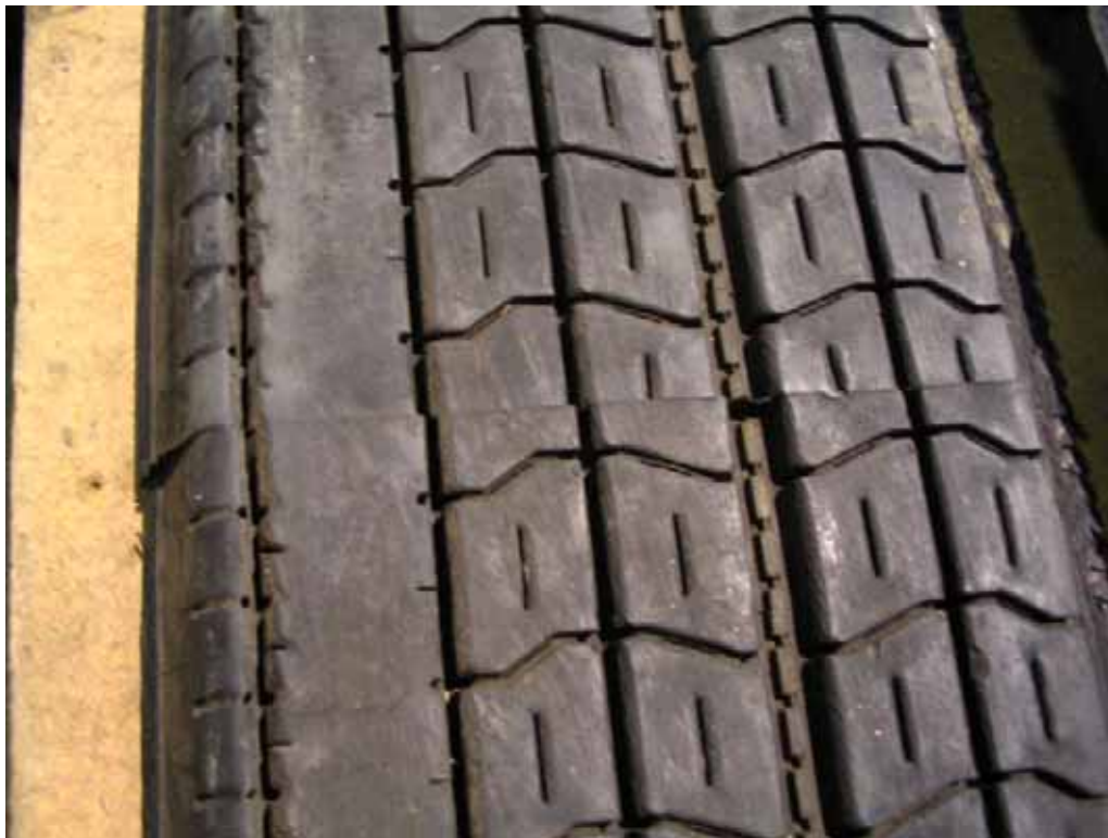
Figure 5.4 – Misaligned Splice on a Pre-Cure Retread Casing
