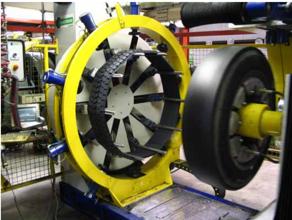
Figure 2.12 – Application of New Tread (Ringtread Process)
