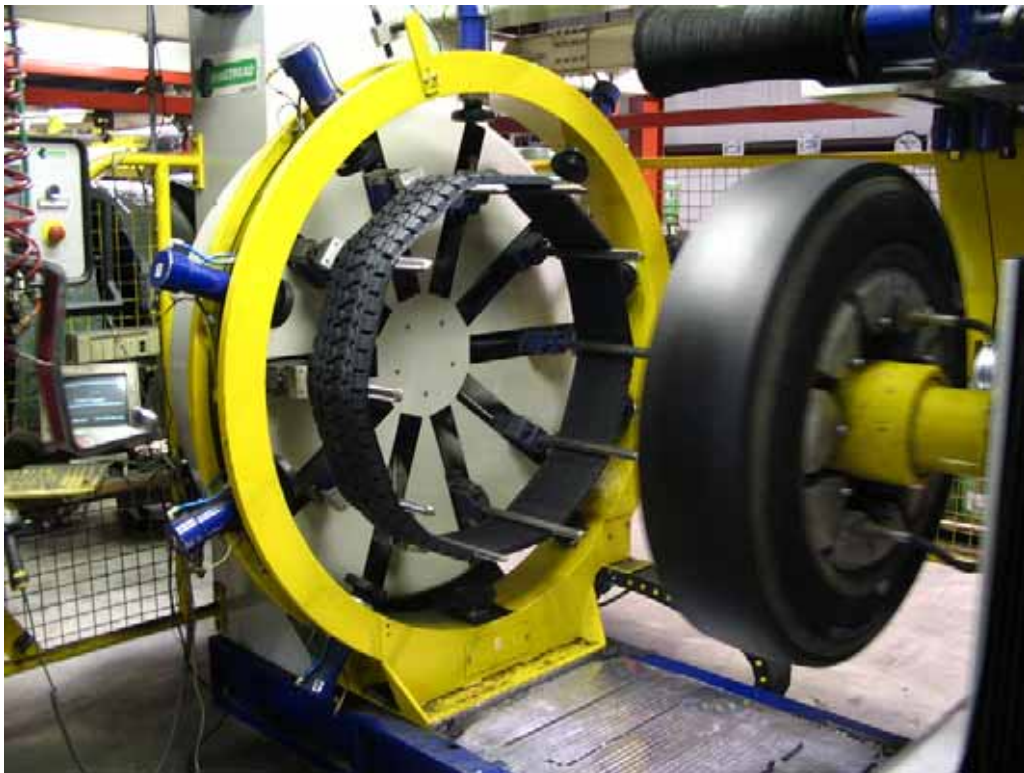
Figure 2.22 – Precured Tread (Unbroken) Stretched to Receive Casing (Ringtread process)
