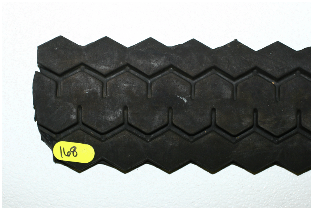
Figure 9.17 - Manufacturing/Process Issues #3 - Bond failure at buff line
