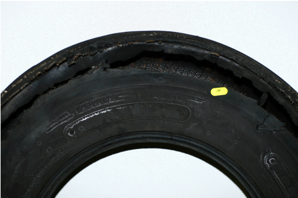
Figure 9.5 - Excessive Heat #2 (Original tread with very significant heat damage (bright bluish discoloration), including localized reversion of rubber)
