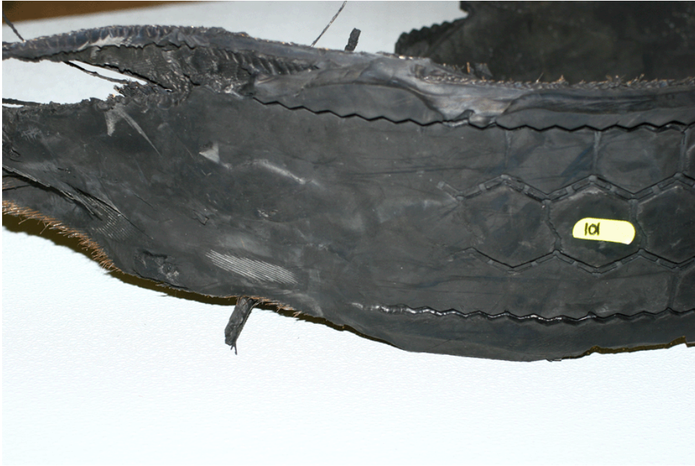
Figure 9.14 – Maintenance/Operational #3 - Example of drive axle tire with localized accelerated wear
