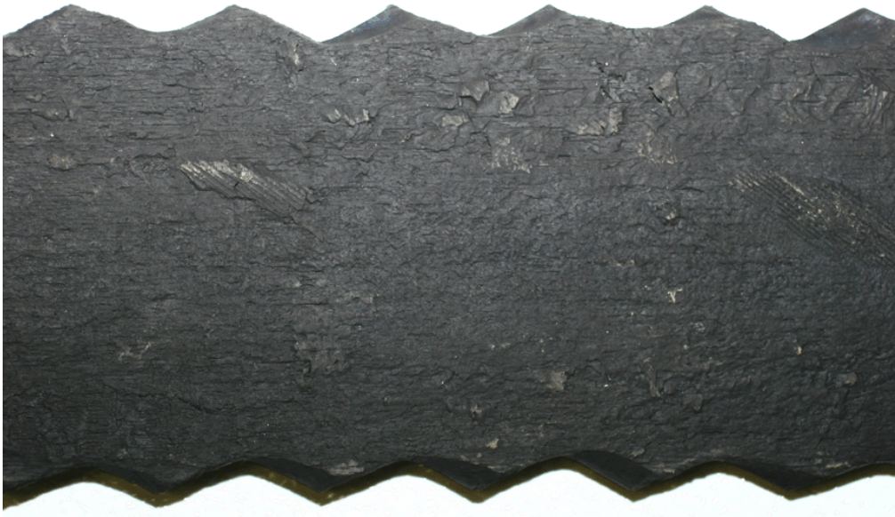
Figure 9.18 - Manufacturing/Process Issues #4 - Bond failure at buff line
