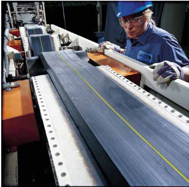
Figure 2.17 – Uncured Rubber (Mold-Cure Process) Courtesy of Bridgestone Firestone
