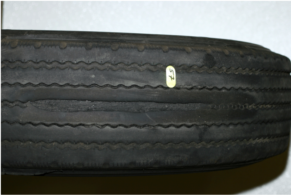
Figure 9.16 - Manufacturing/Process Issues #2 - Retread rubber separated at buff line. This resulted in a "raised" section of the tire's circumference. Localized, accelerated wear (9" in the center of the tread) resulted, extending to the buff line.
