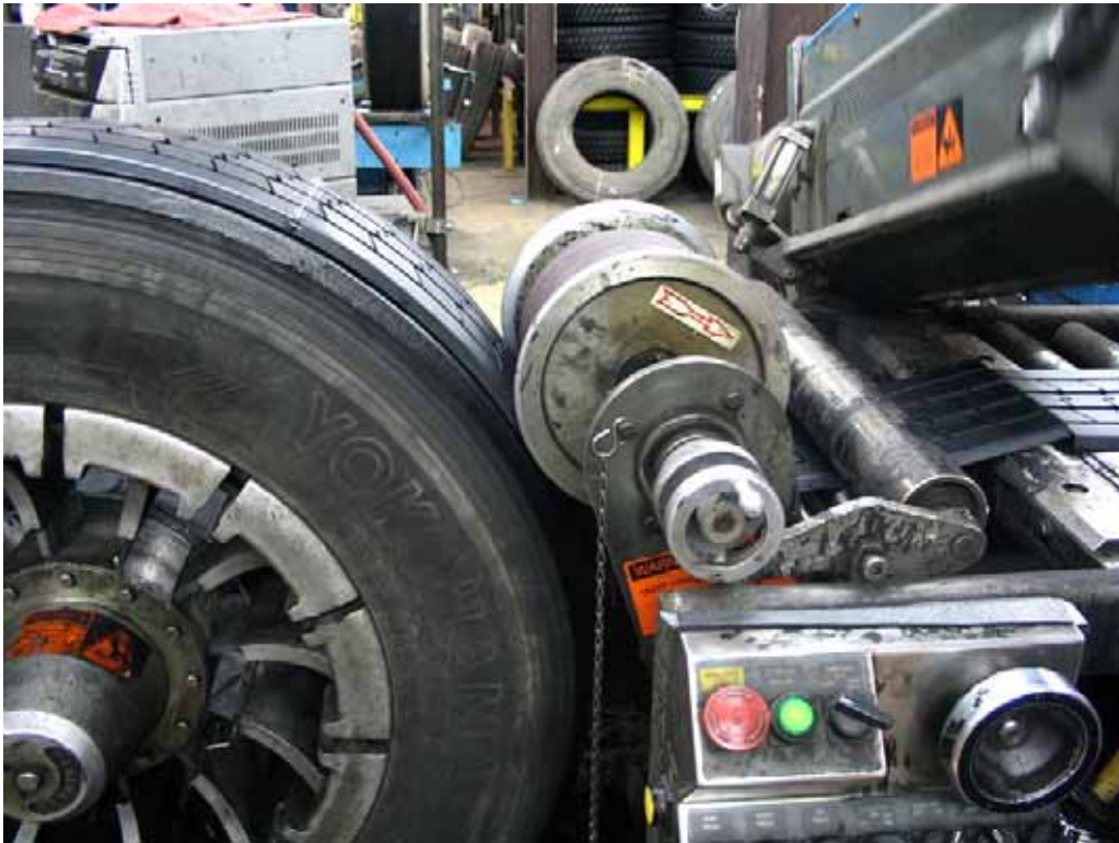
Figure 2.11 – Application of New Tread (Precure Process)
