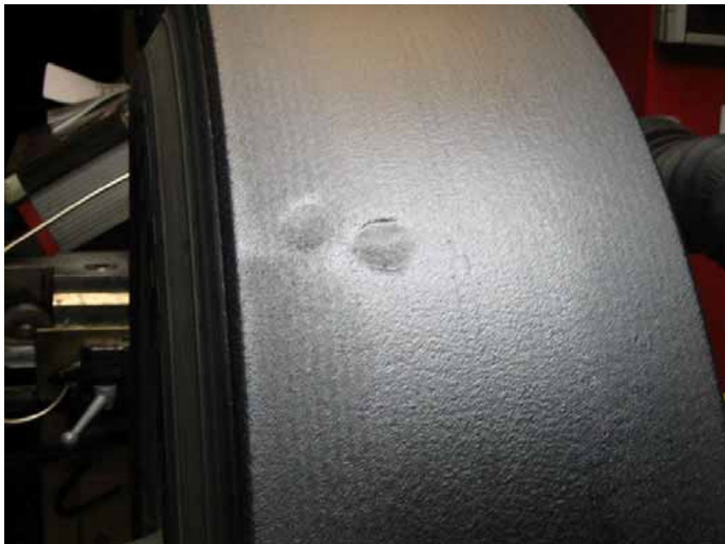
Figure 2.10 – A Buffed Casing After Required Repair
