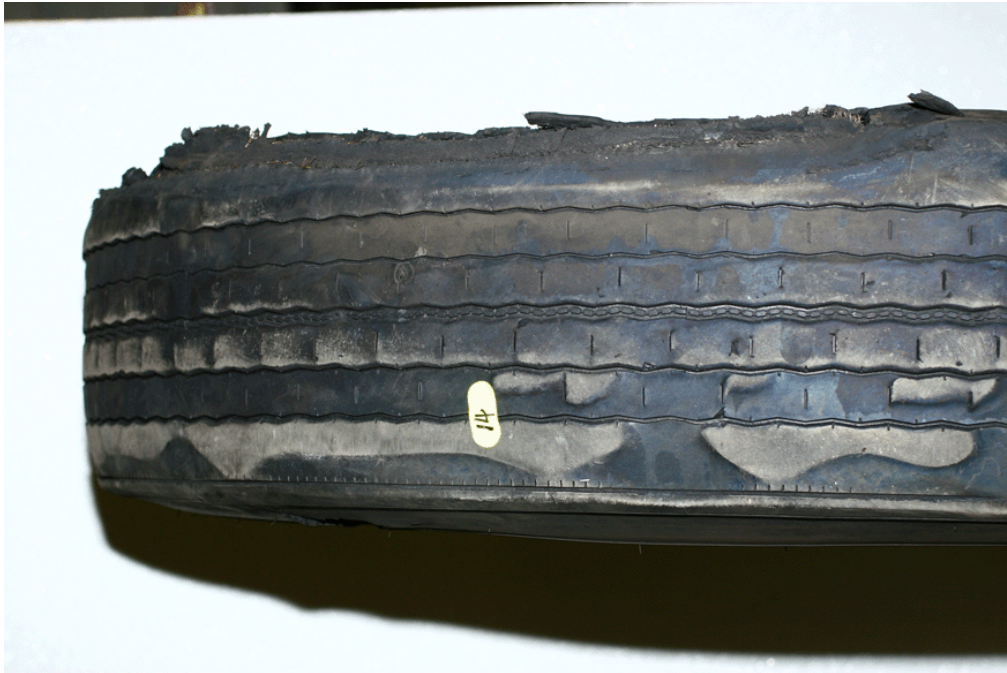
Figure 9.4 - Excessive Heat #1 (This overdeflected tire showed vibrant bluish discoloration, characteristic of operating at excessive temperatures)
